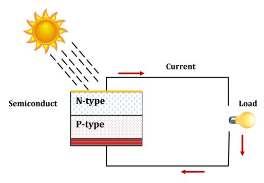
Figure A1.7: Photovoltaic Effect (Mechanical Engineering, 2013)
