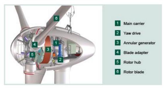
Figure A1.3: Gearless Wind Turbine (Enercon GmbH, 2014)
