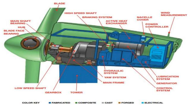
Figure A1.2: Geared Wind Turbine Schematic (AWEA, 2011)
