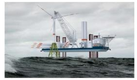
**Figure A13.1:** Wartsila high performance turbine installation vessel
