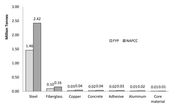
Figure 4.3: Wind Turbine Material Requirements up to 2017
