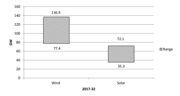
Figure 4.2: Technology Wise Estimate of the Installed Wind and Solar Capacity (in GW) During 2017-32
